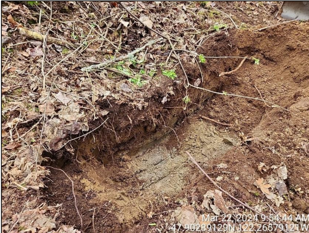
Image of TP-7 excavated to 3 feet below ground surface (bgs).
